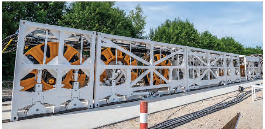
The innovative Bauer Cube System could open up entirely new opportunities for the future construction of diaphragm walls. The system has been developed precisely with container dimensions, meaning it can be used without any problem in microtunnels with small diameters.
