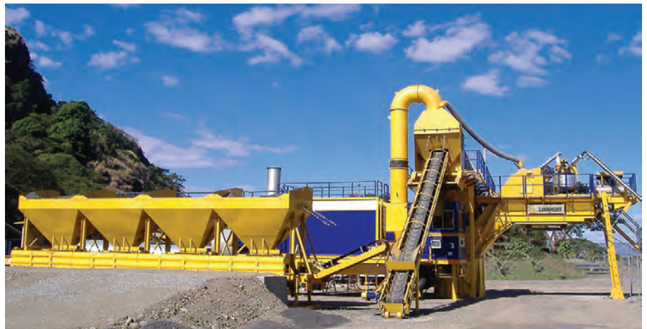
ABOVE AND LEFT: With their fast mobilisation and no need for heavy cranes for installation, Linnhoff TSD 1500 MobileMix asphalt plants can be swiftly relocated to other sections of the highway as required.
