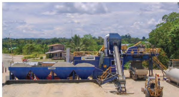
ABOVE AND LEFT: With their fast mobilisation and no need for heavy cranes for installation, Linnhoff TSD 1500 MobileMix asphalt plants can be swiftly relocated to other sections of the highway as required.
