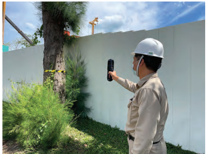
TOP AND ABOVE: The 3D reality capture technology enables users to replicate the on-site environment and turn this into virtual 3D models that can be viewed and accessed remotely.
