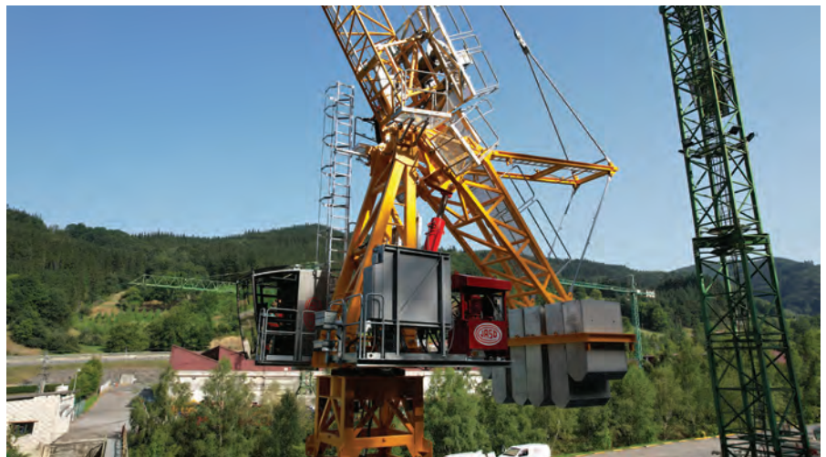
TOP AND ABOVE: The new Jaso IJ198HPA hydraulic luffing tower crane features a maximum load of 18 t. This model is suitable for urban projects or high-rise construction in congested inner cities.
