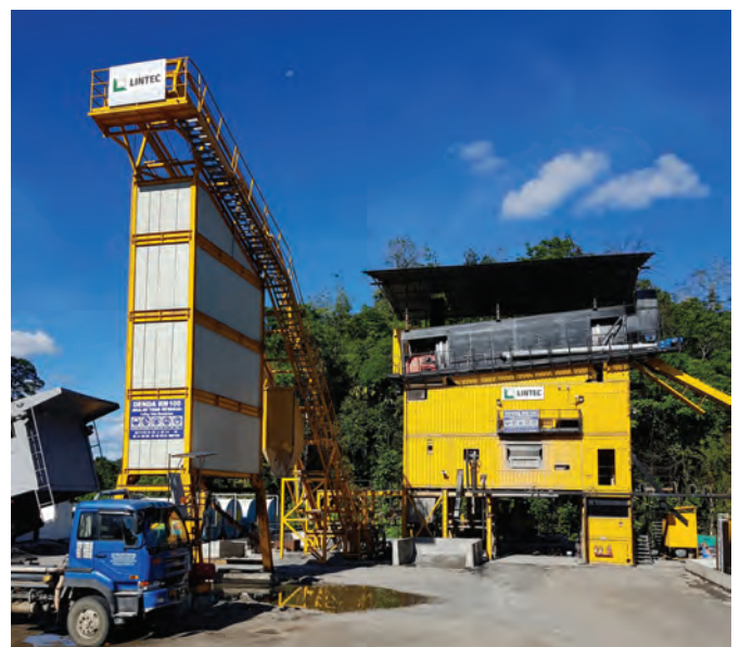
Lintec CSD 3000 (pictured) and CSD 2500B containerised asphalt plants can produce up to 240 t/hr and 160 t/hr respectively. They are equipped with large hot mineral bin capacities to ensure steady batch production.
