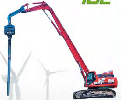
Excavator Vibro Hammer
